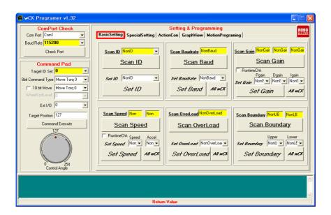
4 Match the Com Port with actual Control Box connected COM Port, then press Scan Baud button, it shows "wCK configured comm. speed" in Scan Baudrate.
